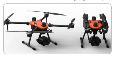
• The Aquila-3F drone by ARGOSDYNE is a versatile and customizable solution for construction, law enforcement, and mapping applications. It offers stable flight performance, a long flight time, and foldable arms for easy transportation and space-saving. The drone's self-designed components and software allow for tailored configurations. It comes equipped with various cameras, searchlights, and speaker systems.
